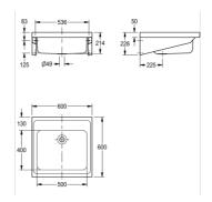
A single bowl sink manufactured from 1.2mm thick, grade 1.4301 (304) stainless steel, satin polish finish. The sink top is turned down on all four edges and incorporates a wet area recess. The bowl is prepared for a 38mm waste outlet.
